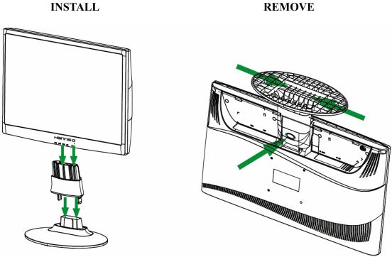
Figure.1. Installing and Removing the Base
